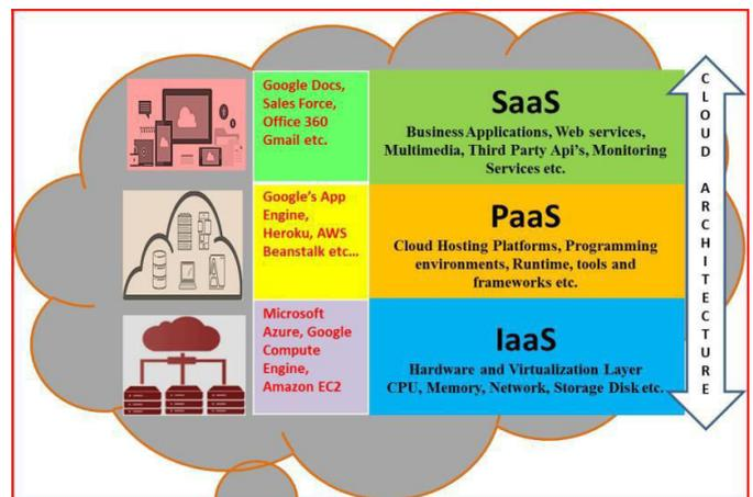
Figure 6- Cloud Computing Service Layers Architecture
