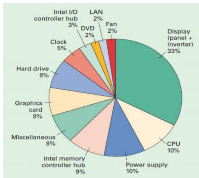
Figure 1- Power Consumption of average lap top
