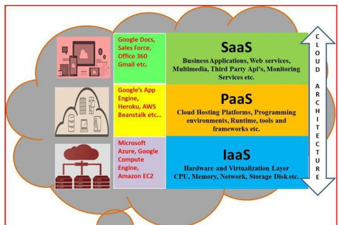
Figure 6- Cloud Computing Service Layers Architecture
